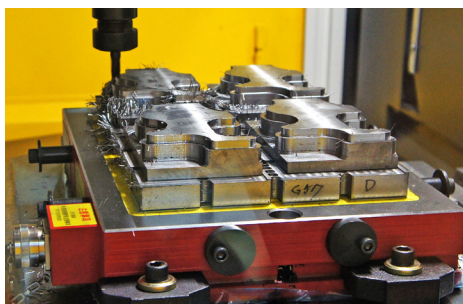
Gang part setups together and still machine 5 sides
